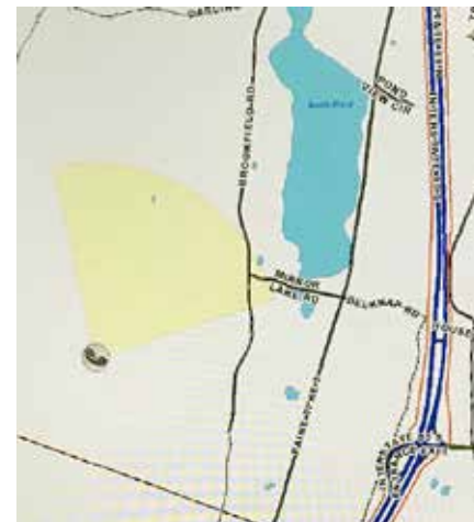
A phase one map shows the shadowed area of coverage near the tower closest to a wireless 911 caller.
