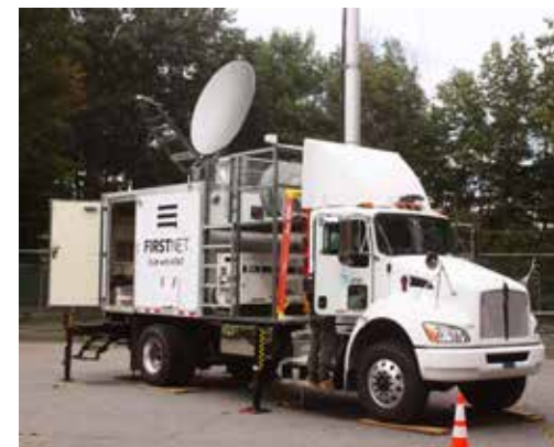
Vermont was the first state in New England to receive an AT&T SatCOLT built for public safety under the FirstNet contract. The unit is stationed at the AT&T facility in South Burlington.
